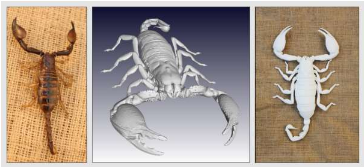
Figure 2: Opisthophthalmus carinatus (Robust burrower) production process. From left to right: Wet specimen (approximately 100mm), STL image, Nylon print (350 mm).
