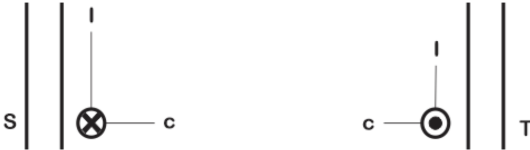
Figure 7: When the current in S creates a transverse electric field (electrodynamic), the field induces a force on T , thereby creating a current. The induced current depends on the distance, which by the model depends on the field density \beta .
