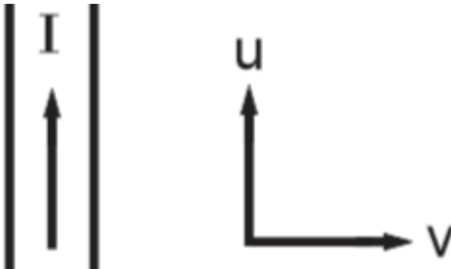
Figure 4: For every outflowing fluid from the linear configuration, there is a perpendicular velocity \mathbf{u} equal to and produced by the motion of the current. This gives the flow two components: The default longitudinal component and the current's motion-induced transverse component.
