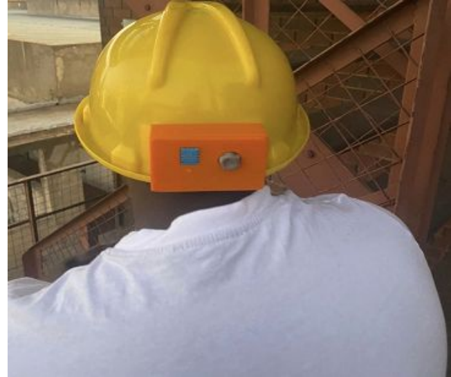
Figure 4: Field testing of smart helmet in mineshaft.
