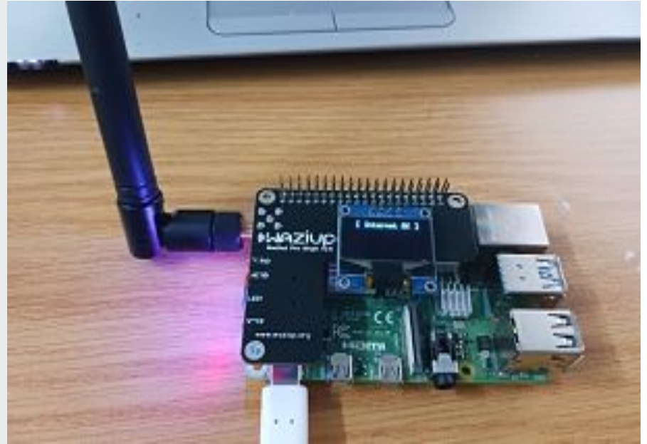
Figure 2: Gateway built using Raspberry Pi and LoRa hat.
