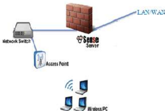
Fig 2.2: Topology of PfSense installation on the LAN (Source: Developed by researchers)
